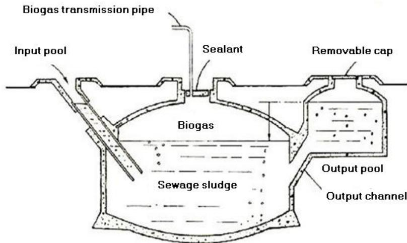
Fig. 4. The components of a biogas generator device [1]
